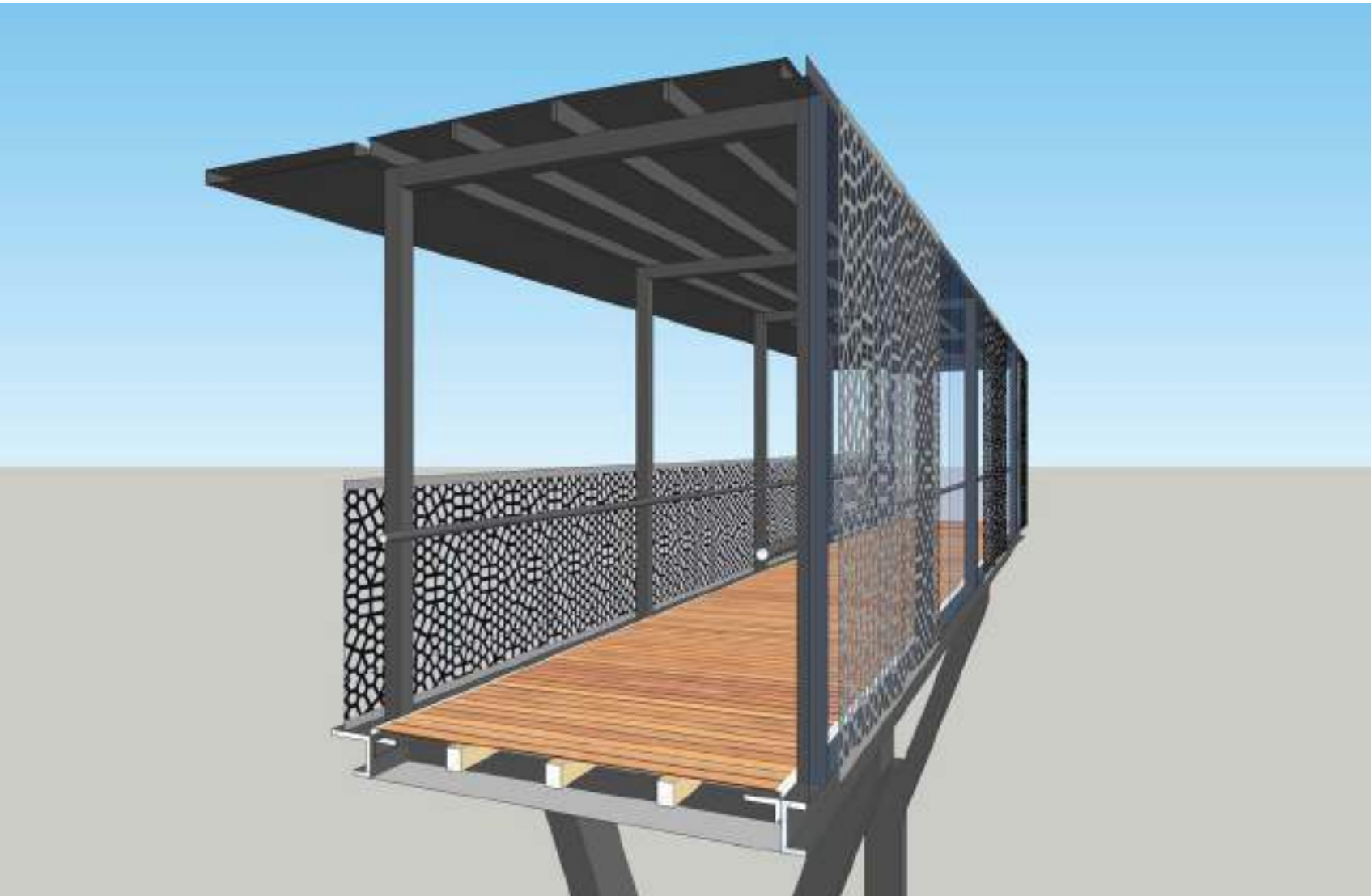
PERFORATED ALUMINIUM SCREEN TO EXTERIOR
